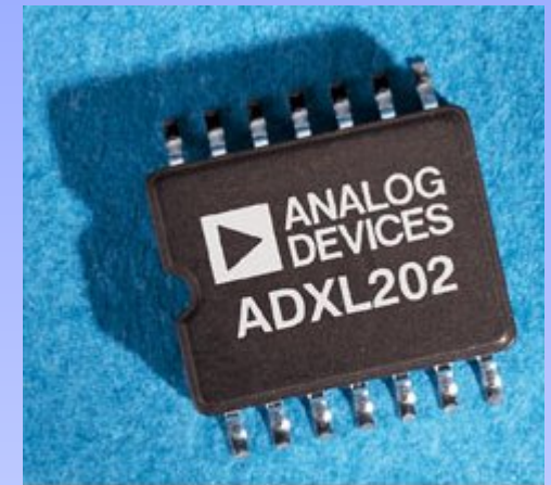
Figure 6. iMEMS accelerometer in surface mount package
