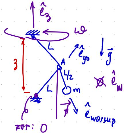
$$\begin{aligned} \vec{\omega}' &= \vec{\omega} + (-\dot{\phi}) \hat{e}_N \\ &= \omega \hat{e}_3 - \dot{\phi} \hat{e}_N \end{aligned}$$
