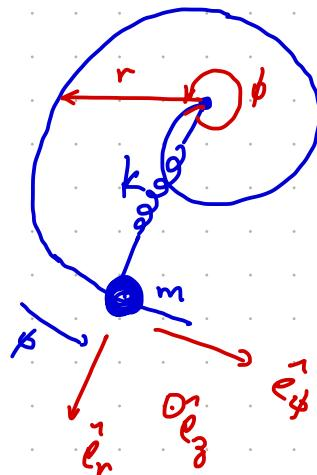
$$\frac{\partial \mathcal{L}}{\partial r} = m\ddot{r}(1+4\pi^2r^2) \Rightarrow m\ddot{r}(1+4\pi^2r^2) + m\dot{r}(4\pi^2r\dot{r})(2)$$
